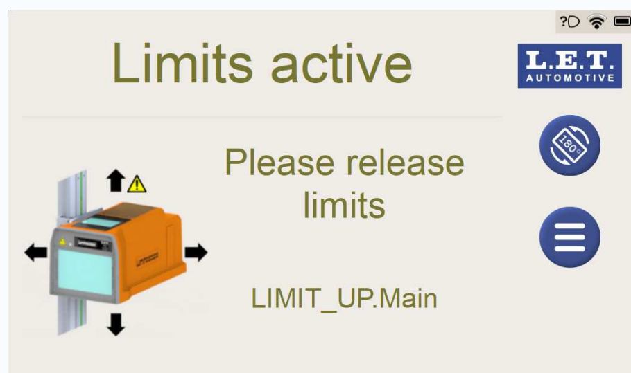
Figure 47: Hardware limit switch active at the highest position for the vertical movement.
