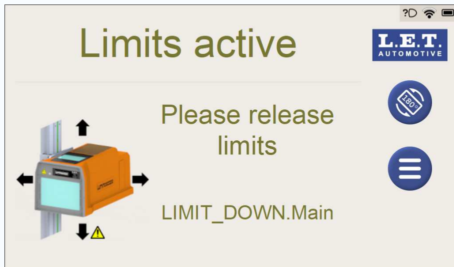
Figure 48: Hardware limit switch active at the lowest position for the vertical movement.
